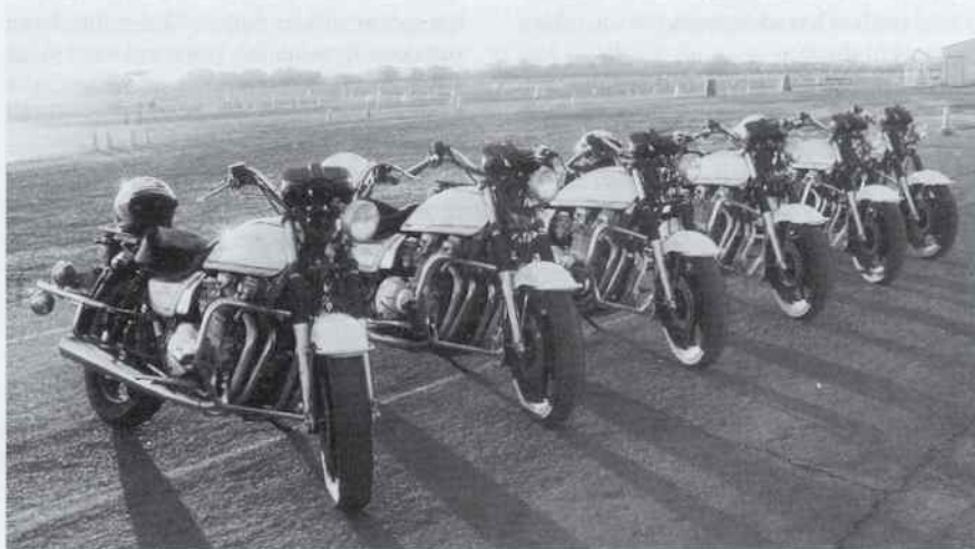
Photo 2: Six training bikes await the first day's lessons at dawn. These bikes have been retired from active patrol duty and are stripped of the sirens, lights, windshields, fairings and heavy saddlebags full of radio equipment that standard police bikes have. Training will be hard on them.
